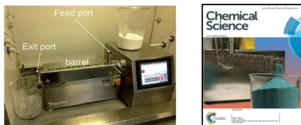
Figure 2. A twin-screw extruder used for scalable solvent-free production of MOFs and other materials.
